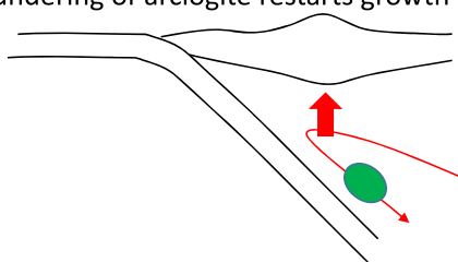
Fig. 2 (Color online) Cartoon showing how arc crust magmatically thickens. In a , subduction drives corner flow in the mantle wedge (red line), leading to decompression melting (large red arrow). These melts rise and intrude or underplate the over-riding plate, causing the crust and associated deep crustal mafic cumulate pyroxenites (green) to thicken ( b ). Dense pyroxenite layer eventually reaches a critical thickness after which it founders into the mantle wedge ( c ). Continued melting in the mantle wedge, provided subduction continues, re-initiates the cycle of arc crust growth
