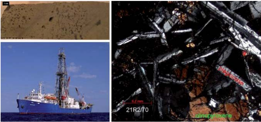
Fig. 1: (A) Photograph of an ODP (Leg104 642E) MORB core sample from the N Atlantic, and (B) Cross polarized light microphotograph of a typical tholeiitic MORB from the N Atlantic (C) Photo of the unique IODP scientific research vessel Joides Resolution, specially designed to drill deep into the sea floor (Photo C from www-odp.tamu.edu ).
