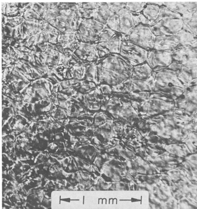
Fig. 1. A view parallel to the c -axis orientation of the ice platelets in ice containing 2% NaCl.
